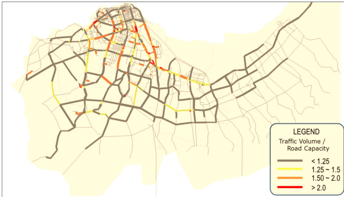
Figure 7.6.6 Highway Assignment Results of Road Intensive Scenario in 2030
