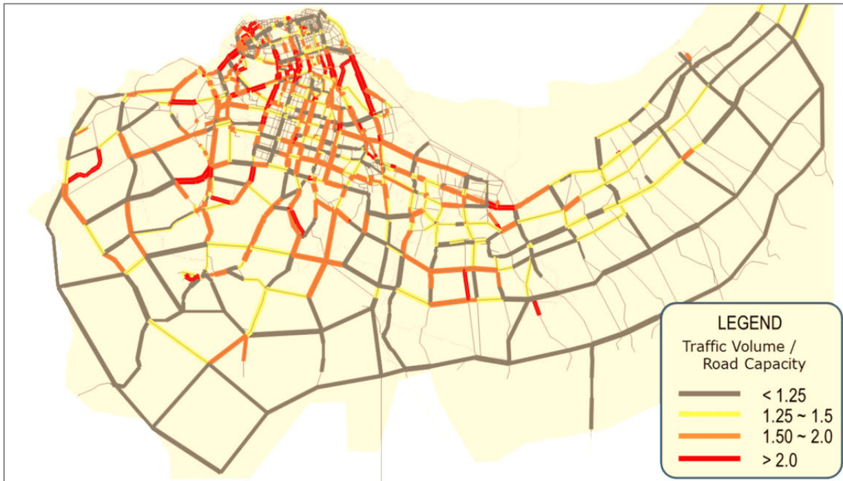
Figure 7.6.10 Highway Assignment Results of Road Intensive Scenario in 2040
