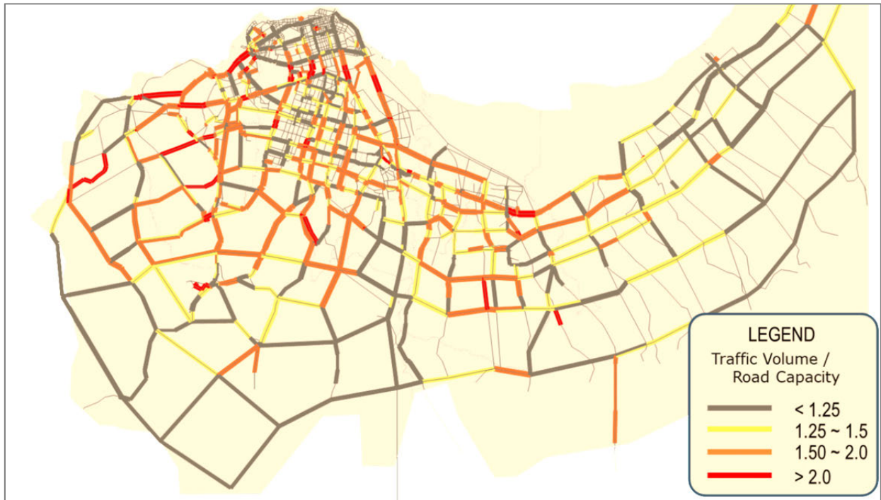
Figure 7.6.14 Highway Assignment Results of Public Intensive (Rail) Scenario in 2040
